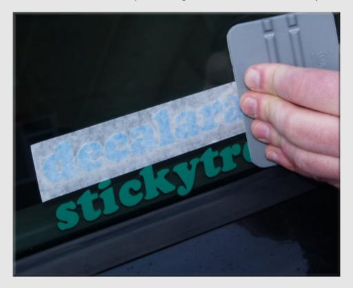
The application tape/paper can now be removed. We always advise customers to pull from a top corner and if possible diagonally across (as shown in the photograph below).
